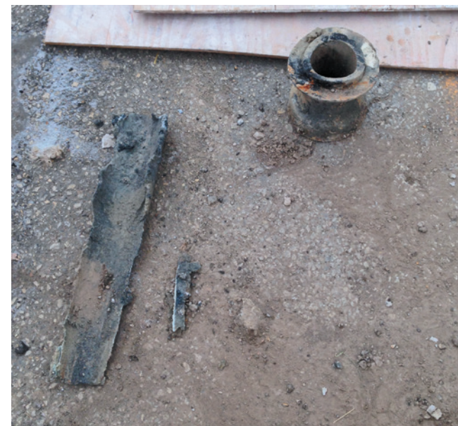
The excavated remains of a disintegrated sewer connecting line.
